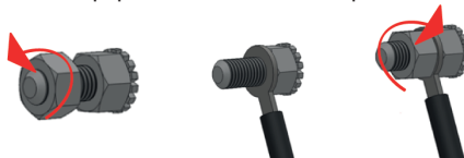
Figure 4. Connecting the unit to an electrical equalizing system.
